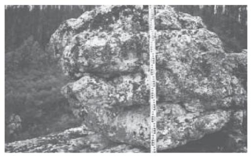
Photo 6. Boulder affected by selective weathering through sub-horizontal joints .
