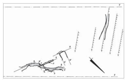
Figure 3. Endo and exokarstic forms and fractures (GROBA & VAQUEIRO, 2003). F: Marginal fault (Y), N135°E-N140°E; R-fractures: N110°E; R'-fractures, N20°E; P-fractures, N160°E; T-fractures, N55°E.
